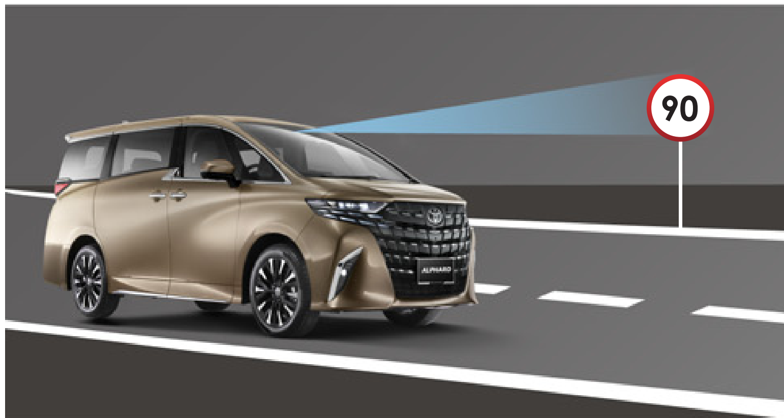
ROAD SIGN ASSIST (RSA) Monitors the road ahead, displaying information such as current speed limit and suggesting necessary adjustments.
