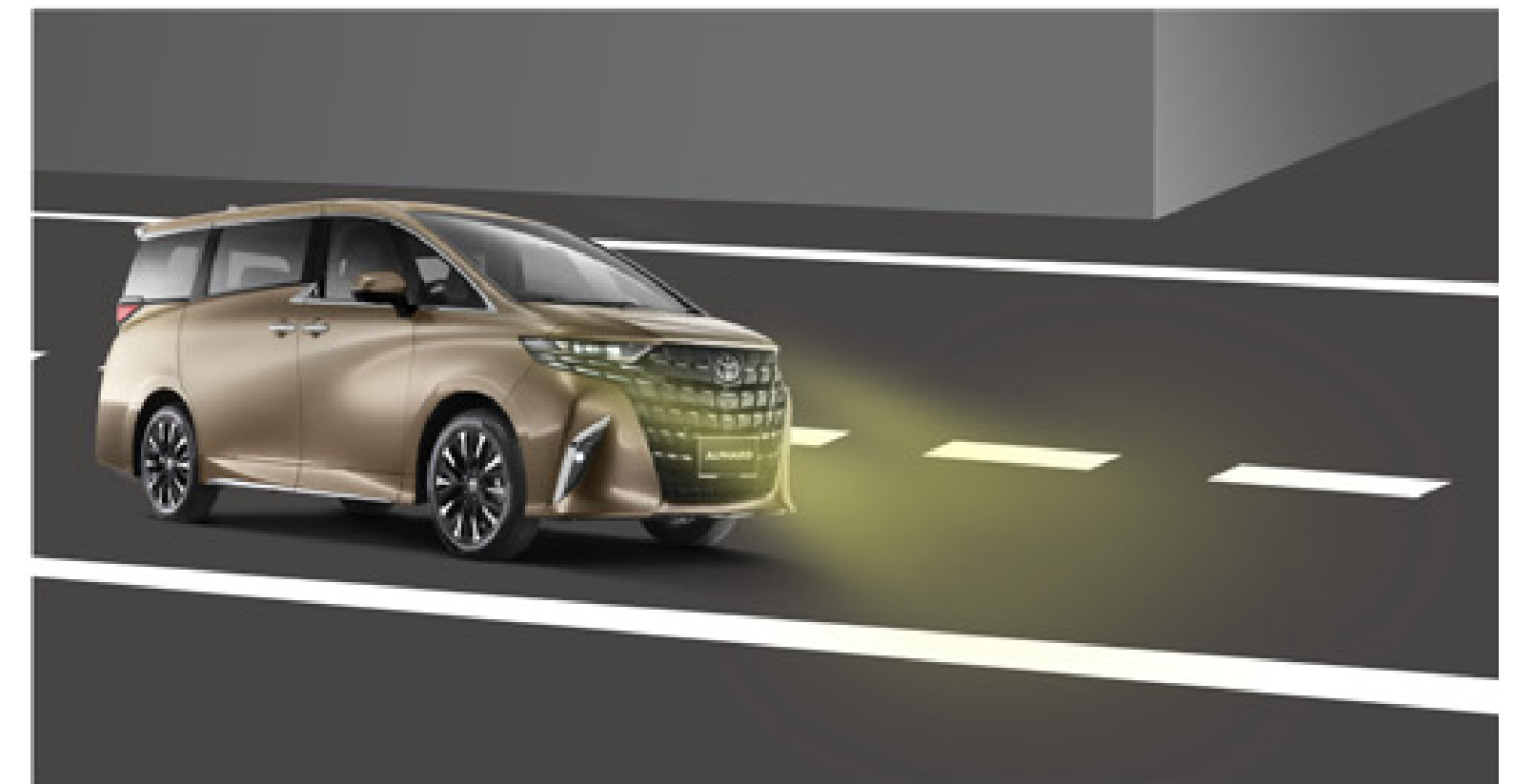
ADAPTIVE HIGH BEAM SYSTEM (AHS) Automatically adjusts the auto high beam headlight distribution to not illuminate directly on oncoming vehicles.
