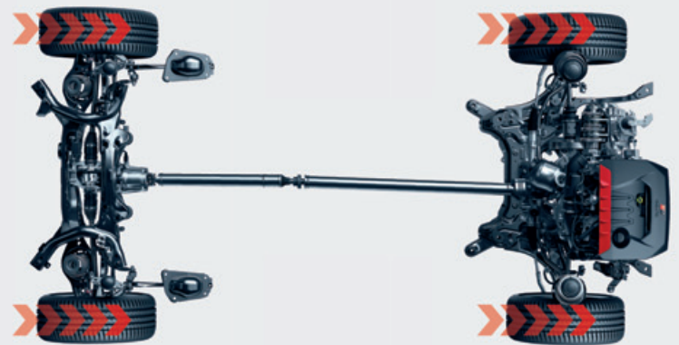
TRACK mode [Front wheel 50: rear wheel 50]
